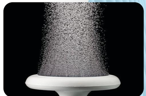
C.L. Smith Industrial's performance blue Filtros **Porous Ceramic** plates are excellent for fluidized beds and an excellent alternative to cloth/fabric air slide material. Air is blown under the ceramic plate, diffusing it and the material above has minimal friction between particles which causes it to act like a liquid.
